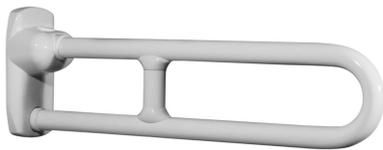
Folding side safety support reinforced with a joint, made of seamless zinc-plated steel pipe, coated with antimicrobial, biocompatible and warm-to-the-touch vinyl
