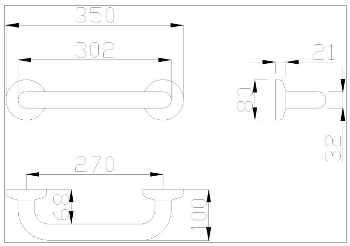
Straight grab bar made of seamless stainless steel AISI 304 pipe, with polished finish
