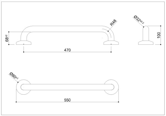
Polished stainless steel straight safety grab rail,  $\emptyset$  32x1.5 mm in AISI 304 stainless steel, no junctions.
