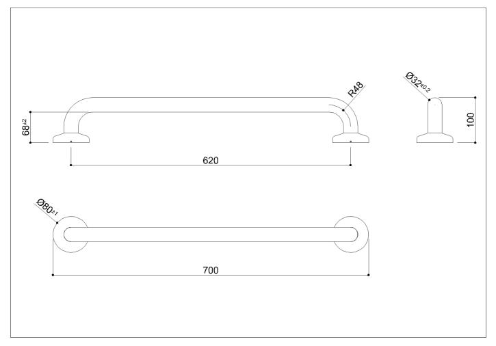
Polished stainless steel straight safety grab rail, Ø 32x1.5 mm in AISI 304 stainless steel, no junctions.
