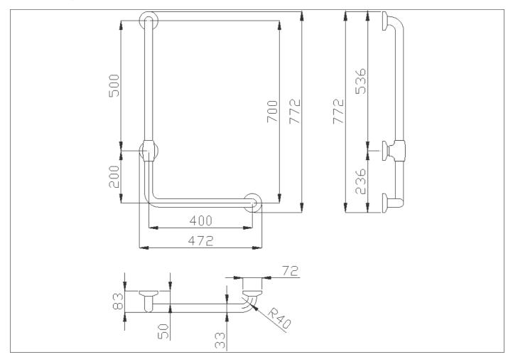
L-shaped grab bar made of zinc-plated steel pipe, coated with antimicrobial, biocompatible and warm-to-the-touch vinyl
