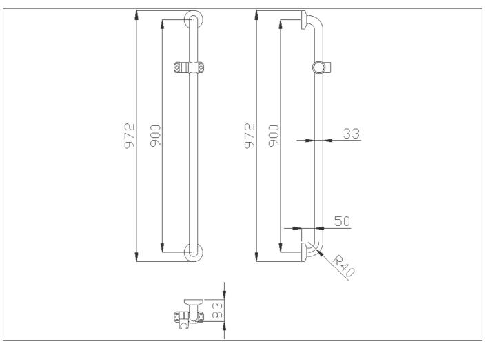
Straight grab bar made of seamless zinc-plated steel pipe, coated with antimicrobial, biocompatible and warm-to-the-touch vinyl. Equipped with hand shower holder
