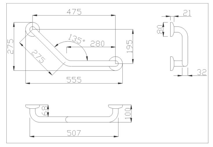
$135^\circ$  angled grab bar made of seamless stainless steel AISI 304 pipe, with polished finish
