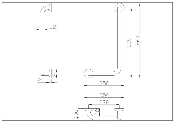
L-shaped grab bar made of seamless stainless steel AISI 304 pipe, with polished finish
